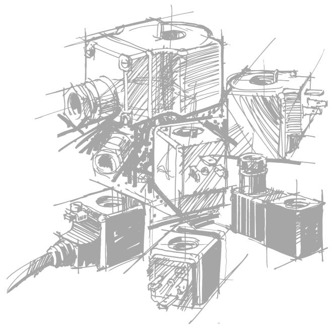
Coils for solenoid valves
